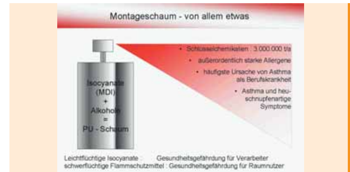
10 Problemstoff Montageschaum (Institut peridomus, 2002)
