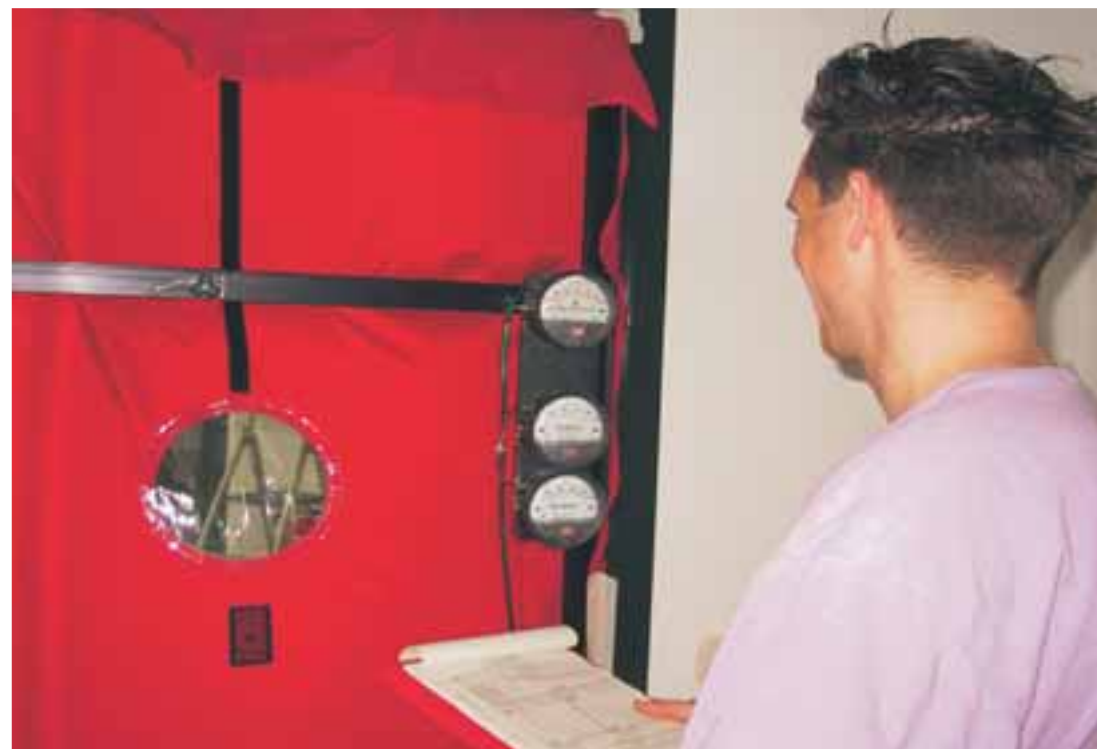
4 Blower-Door-Test: Ablese der Messwerte
